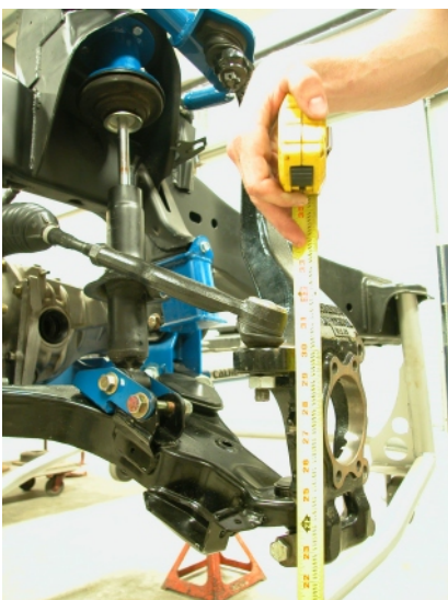
Titan Arm, stock shock mounted in new location with the WTCB. Fully drooped is 30.125" at steering arm to ground. This right at maximum misalignment angle of the new Titan outer tie rod end upgrade. In other words, this is all of the travel you can get out of this without beginning to go to custom parts. Many of which, are not street legal in some states.
