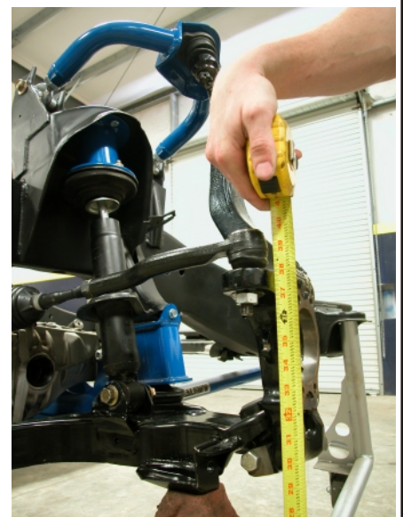
Titan Arm, stock shock mounted in stock location. Fully compressed is 38.000" at steering arm to ground. 5.375" of total wheel travel.
