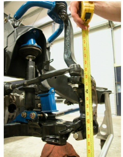
Titan Arm, stock shock mounted in new location with the WTCB. Fully compressed is 37.875" at steering arm to ground. 7.75" of wheel travel with the new shock bracket. 44% plus increase in wheel travel at the knuckle.
